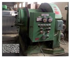
Fig (1): Shot peening machine with shot balls.
