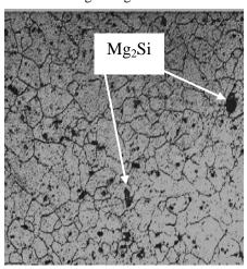
Fig (3): Show the microstructure of metal, 500X.
