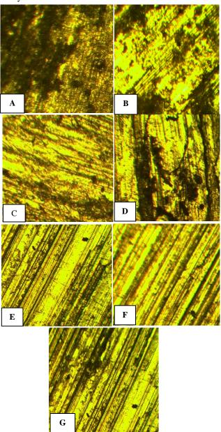
Fig (7): Optical Surface morphology of Al- Alloy 6061-T6 specimens (500X), A: as received and B, C and D corrosion in sea water. E, F and G corrosion in tap water.
