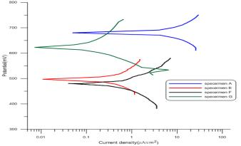
Fig (6): Polarization curves for specimens in tap water media.
