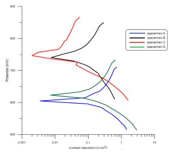
Fig (5):Polarization curves for specimens in sea water media.
