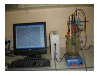
Fig (2): the electrochemical corrosion unit.
